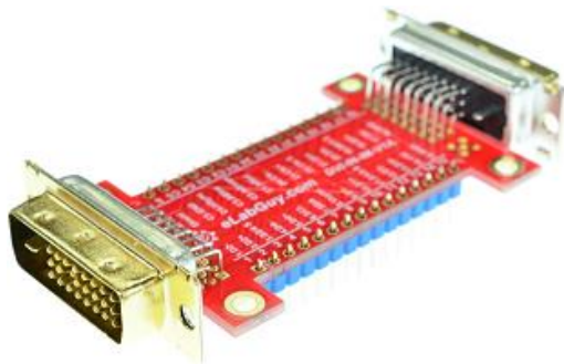
Figure 3: DVI-DM-DM-V1A with headers
